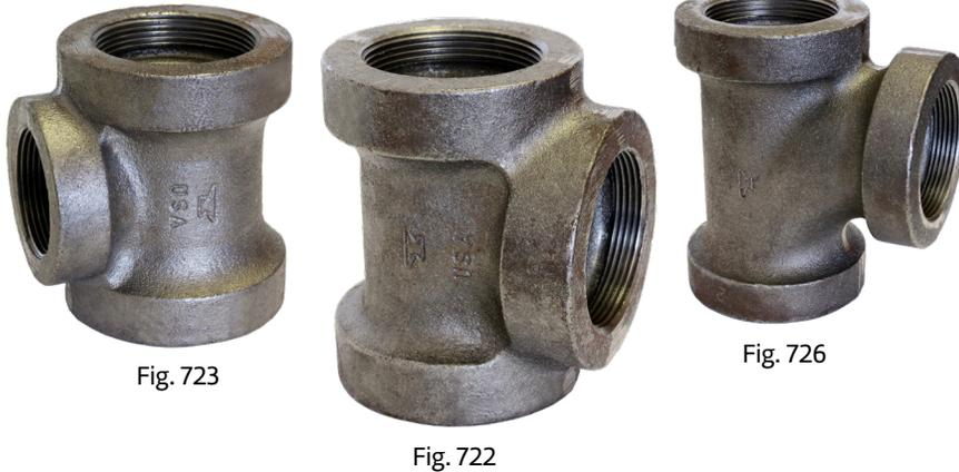
Anvil drainage fittings have sufficient sweep to allow free unobstructed flow. They are made with a shoulder of the same diameter as the inside of the pipe, in accordance with ASME B16.12, Type 1. Thus, continuous passage is created when the pipe is screwed to the shoulder, leaving no place for solid matter to collect and clog in the pipe.
